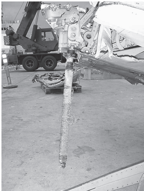
Figure 1. Jackscrew from Flight 261 Horizontal Stabilizer (NTSB)
